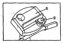
the Resistance Knob clockwise; to decrease the resistance, turn the Resistance Knob counterclockwise.
