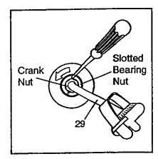
in one of the slots in the slotted bearing nut. Lightly tap the screwdriver with a hammer to turn the slotted bearing nut counterclockwise until the arms are po longer loose. Do not overtighten the slotted bearing nut. When the slotted bearing nut is properly tightened, tighten the crank nut.
