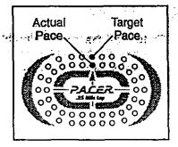
will change periodically during the 18 MPH/90 RPM and 12 MPH/60 RPM programs; as the target pace changes, simply adjust your pace to keep both indica-
