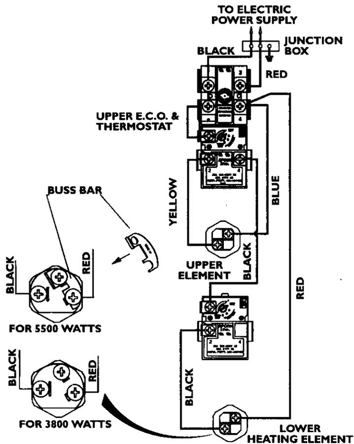
WIRING FOR 3 WIRE LEAD WATER HEATERS
