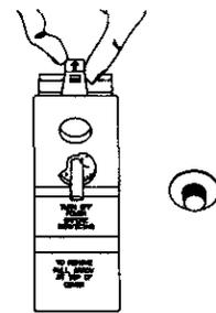
6. Remove the insulation block to expose the opening.
