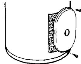
5. After you have removed the lower access panel, remove the adjustment dial from the thermostat by gently pulling it directly away from the thermostat.
