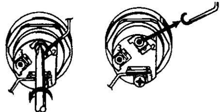
7. The buss bar is labeled 5500 W. Place the buss bar over terminals 2 and 3 with the 5500 W visible. Install the extra screw provided into terminal 3.
