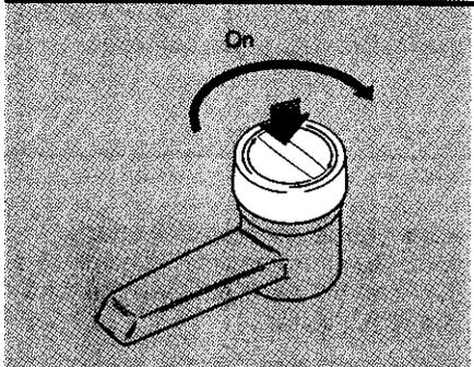
**15.** Push down and turn the On/Off Cap clockwise to open spout. Hold cap open to fill tank (about 1 minute). When tank is full, water will flow from spout. Release cap.
