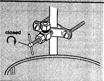
**11.** Turn saddle valve handle clockwise  $\curvearrowright$  until lance pierces soft copper tubing and valve is firmly seated. If the water line is not copper, turn the saddle valve handle clockwise until the valve is firmly seated. The valve is now in the closed position.
