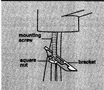
**5.** Loosen square nut until it is flush with end of the mounting screw. Tip spout bracket against mounting screw. (Bracket will form a "y" when in the correct position.)
