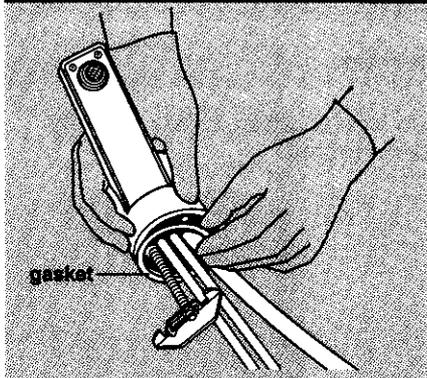
**4.** Lay spout assembly on flat surface with coiled tubing facing up. Using one hand to hold tubing just below spout, carefully straighten
