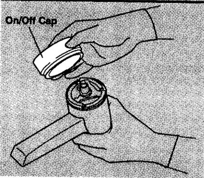
**3.** Remove masking tape and tag from spout assembly. Do Not remove quick-connect fittings from spout tubing or tank tubing. Do not replace quick-connect fittings with brass fittings. Brass fittings can cause lead contamination.
