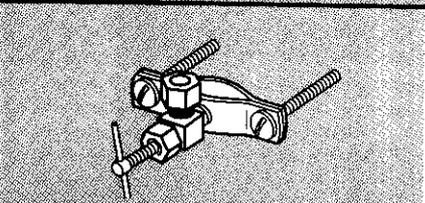
**10.** Install saddle valve following kit instructions. If water supply line is not copper, shut off water supply and
