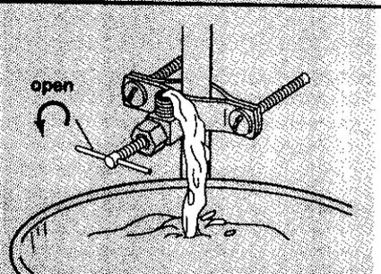
**12.** Slowly open saddle valve and flush line into bucket to remove any foreign material that may have been trapped in the supply line during saddle valve installation. Close saddle valve.
