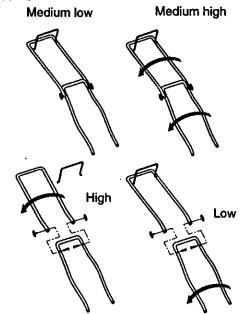
▲ CAUTION: The operator presence control bar must pivot freely to permit blade/ brake engagement when control bar is released. Do not overtighten the fasteners holding the controls to the upper handle.
