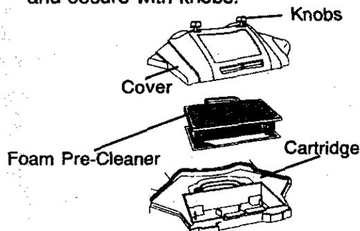
**IMPORTANT:** Petroleum solvents, such as kerosene, are not to be used to clean the cartridge. They may cause deterioration of the cartridge. Do not oil cartridge. Do not use pressurized air to clean or dry cartridge.
