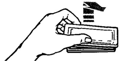
3. Remove the light bulb from its socket. Replace the bulb with another halogen bulb (12 volt, 5 watt maximum, available at most hardware stores).
