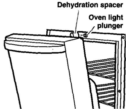
\* The dehydration spacer (Part No. 814166) or the dehydration kit which includes racks and a spacer (Part No. 4395974) can be ordered from your dealer, or by calling 1-800-422-1230 and following the instructions and telephone prompts you hear.
