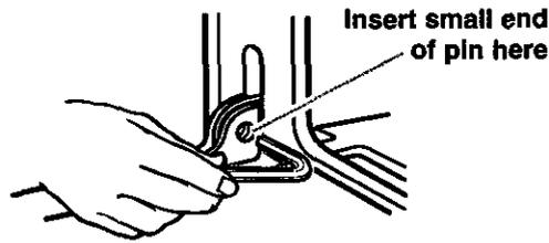
3. Grasp under handle and gently close door as far as it will shut. Pull door out at bottom to remove.
