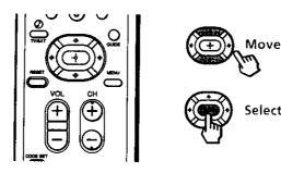
The supplied remote control has "arrow" buttons  $(\spadesuit, \blacklozenge, \spadesuit, \spadesuit)$  which allow for movement of the on-screen  $(\blacktriangleright)$  cursor. Pressing on the outer buttons will cause the cursor to *move* in the corresponding direction. Pressing the center button (+) will *select* the item.
