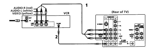
The S-Link connector must be in the same VIDEO-IN column as the connected A/V cables.
