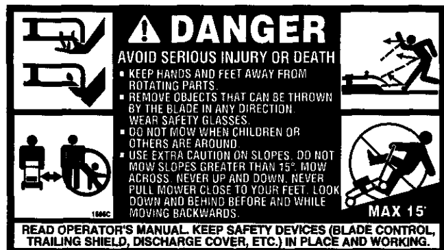
Figure 1 Safety Labels Found On Lawn Mower
