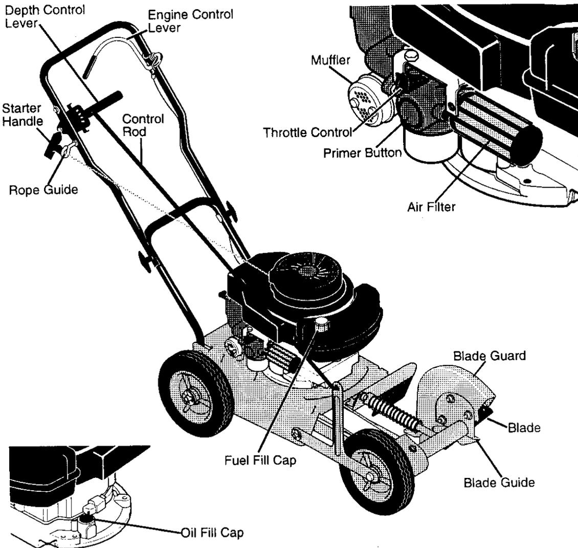
**Throttle Control** – Used to control the engine speed.
