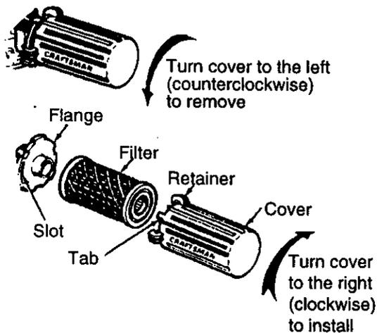
**CAUTION:** Never run the engine without the air cleaner element installed. A defective air cleaner can result in loss of engine power and can cause excessive wear or damage to the engine components if dirt or dust is permitted to enter the engine through the carburetor. A damaged air cleaner, or one that is clogged with dust or dirt should be replaced immediately.
