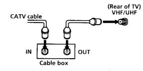
If you are connecting a cable box through the AUX input and would like to switch between the AUX and normal (CATV) input, you should consider using the CHANNEL FIX feature discussed on page 31.
