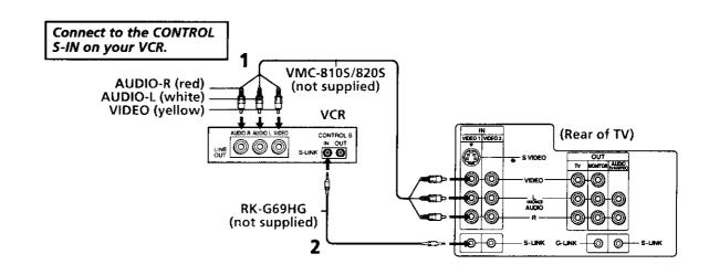
The S-Link connector must be in the same VIDEO-IN jacks as the A/V cables on your TV.
