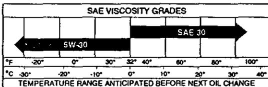
**NOTE:** Although multi-viscosity oils (5W30, 10W30 etc.) improve starting in cold weather, these multi-viscosity oils will result in increased oil consumption when used above 32°F. Check your engine oil level more frequently to avoid possible engine damage from running low on oil. Change the oil after every 50 hours of operation or at least once a year if the tractor is not used for 50 hours in one year.
