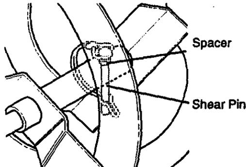
**IMPORTANT:** To ensure safety and performance levels, only original equipment shear bolts should be used. When replacing shear bolts, be sure to replace shear bolt spacers. To replace a broken shear bolt, proceed as follows:
