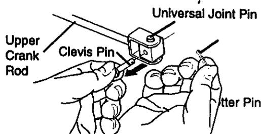
**NOTE:** If this removes the universal joint and universal joint pin. Place universal joint into yoke of upper crank rod lining up large holes. Insert universal joint pin. (Ensure opening in universal joint pin is in line with small openings in universal joint.)
