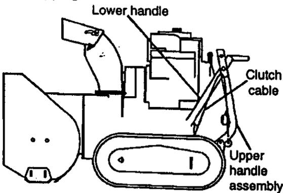
The figure below shows the snow thrower completely assembled. References to the right or left hand side of the snow thrower are from the viewpoint of the operator's position behind the unit.
