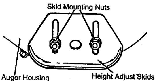
For normal hard surfaces, adjust the skids as follows:
