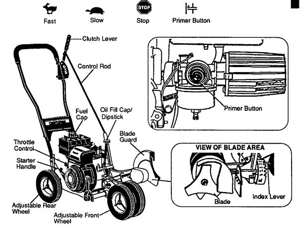
Throttle Control – Used to control the engine speed.
