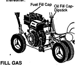
Fill the fuel tank with clean, fresh, unleaded grade automotive gasoline. Be sure that the container you pour the gasoline from is clean and free from dust or other foreign particles. Never use gasoline that may be stale from long periods of storage in the container.
