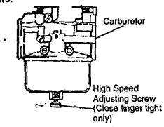
Close the high speed adjusting screw by hand.
