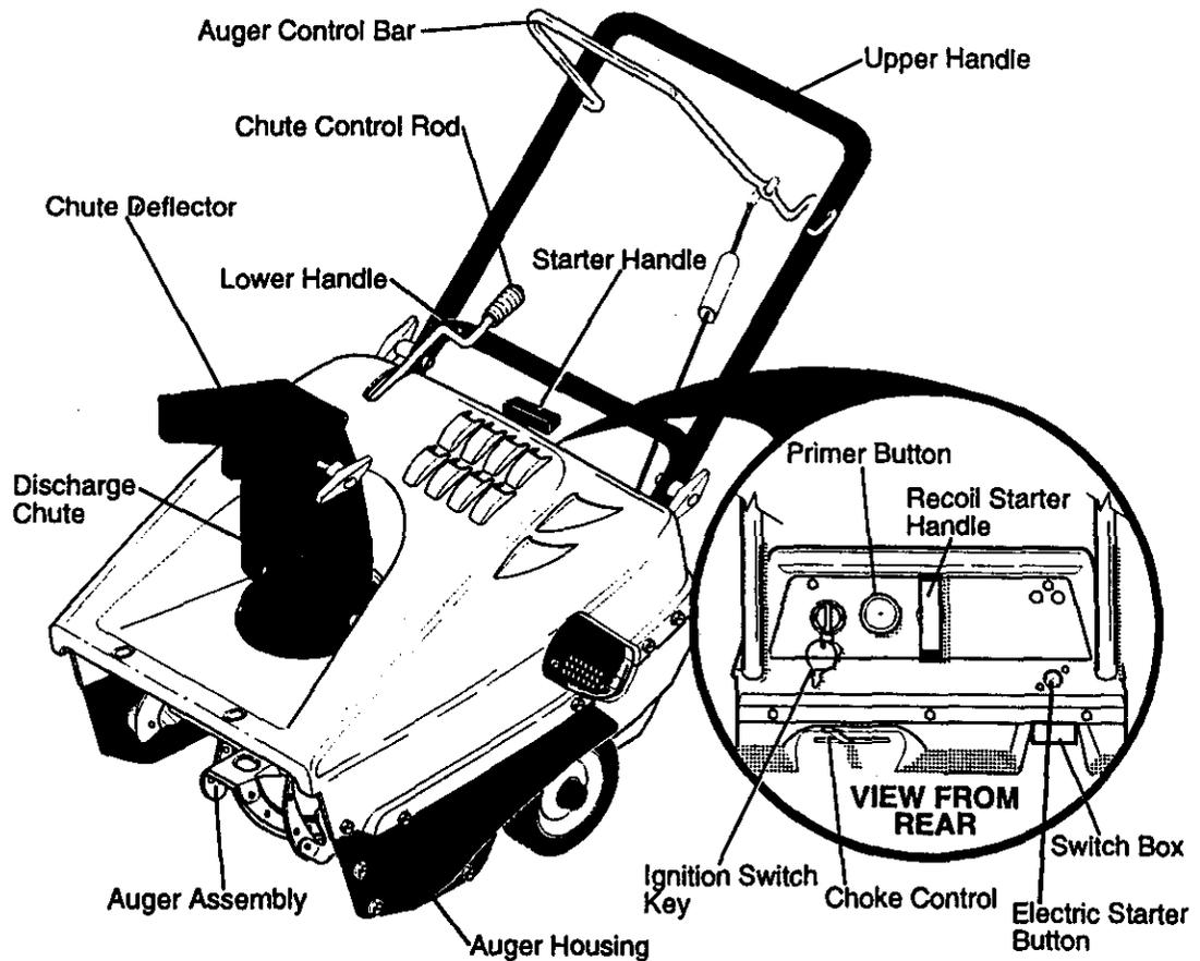
**Auger Control Bar** – Starts and stops the auger which propels the snow thrower.
