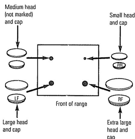
Replace the burner heads on the bases matching the letters. Replace the caps on the heads. Make sure that the caps and heads are replaced in the correct location. There is one small, one medium, one large and one extra large head and cap.
