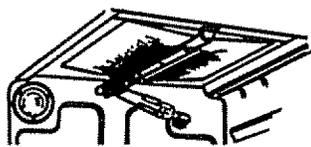
The flames for the top (broil) burner should be steady with approximately 1" blue cones and should not extend out over the edges of the burner baffle.
