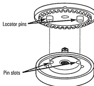
When replacing, make sure the locator pins in the burner head are seated in the pin slots of the burner base. Rotate the burner head around the burner base until it is level and securely seated.
