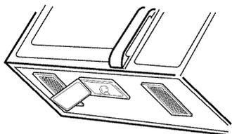
2. **Remove** the bulb cover mounting screws.
