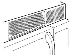
6. **Slide** the bottom of the vent grille into place. **Push** the top until it snaps into place. **Replace** the mounting screws.
