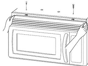
3. **Tip** the grille forward, then lift out to remove.
