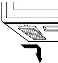
3. Soak grease filter in hot water and a mild detergent. Rinse well and shake to dry. **Do not use ammonia or place in a dishwasher. The aluminum will darken.**
