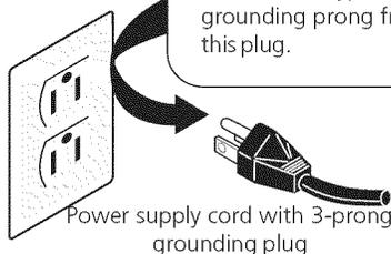
Power supply cord with 3-prong grounding plug
