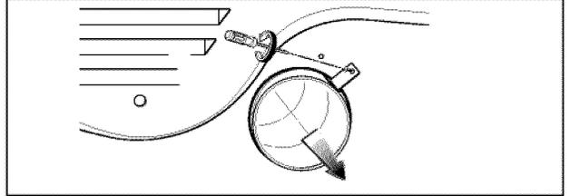
2. Detach and remove the bottom, left or right side knockout as desired.
