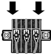
6. Tighten strain relief screws.
