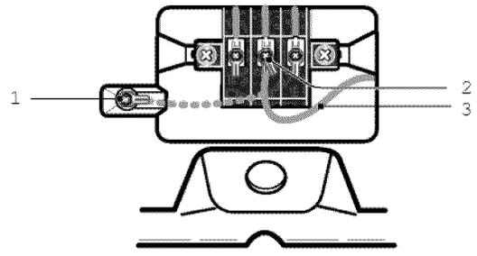
1. External ground connector - Dotted line shows position of NEUTRAL ground wire before being moved to center terminal block screw
