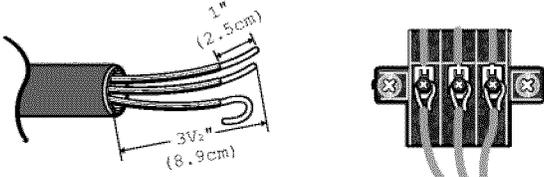
1. Loosen or remove center terminal block screw.
