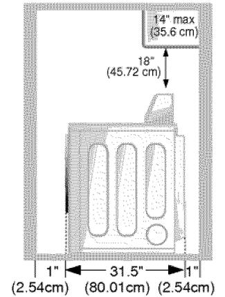
\* Most installations require a minimum 5 1/2 in. (14 cm) clearance behind the dryer for the exhaust vent with elbow.
