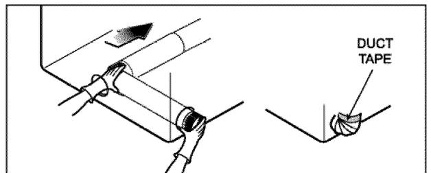
5. Insert duct assembly, elbow first, through the side opening and connect the elbow to the dryer internal duct.
