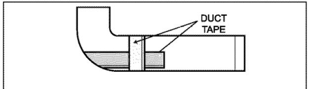
4. Pre-assemble 4" elbow with 4" duct. Wrap duct tape around joint.
