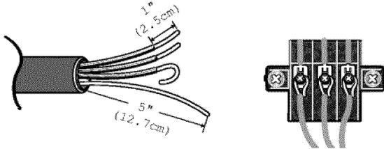
1. Remove center terminal block screw.
