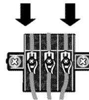
4. Tighten strain relief screws.
