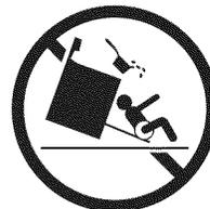
To reduce the risk of tipping, the appliance must be secured by properly installed anti-tip bracket provided with the appliance. To check if the bracket is installed properly; grasp the top rear of the
