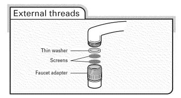
Insert the 2 screens and then the thin washer from the faucet adapter kit into the faucet adapter. Attach the adapter onto the end of the faucet.
