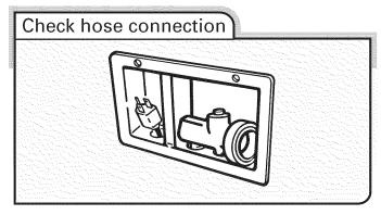
3. Pull down on the locking collar while lifting the hose connector onto the faucet adapter.
