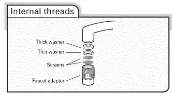
Insert the 2 screens, the thin washer, and then the thick washer from the faucet adapter kit into the faucet adapter. Attach the adapter onto the end of the faucet.
