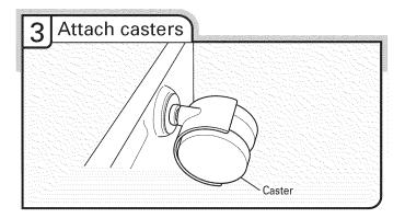
Firmly push casters into holes at corners of dishwasher as shown. Pull on each caster to check that casters are snug.
