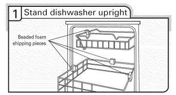
Stand dishwasher upright. Open door and remove shipping foam, cardboard tower and any other shipping materials. Close dishwasher door. Latch dishwasher door shut.
