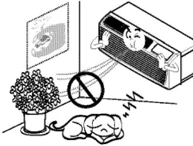
**Do not block the inlet or outlet of air flow.**
