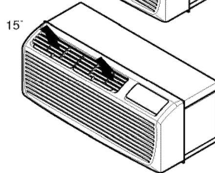
To adjust the air direction, remove the front grille. Remove the 4 screws that fasten the discharge grille to the front grille.
