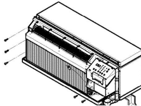
4. Reinstall the front grille by hooking the top over the unit top, then pushing it in at the bottom.
