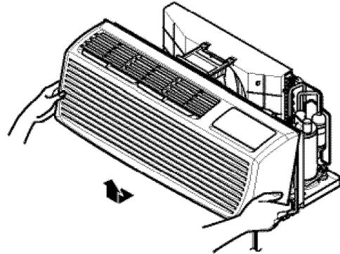
3. Slide the unit into the wall sleeve and secure with 6 screws through the unit flange holes.
