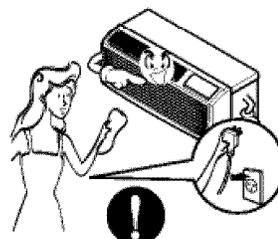
**Turn off the main power switch when not using it for a long time.**
