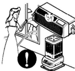
**Turn off the power and breaker when cleaning the unit.**
