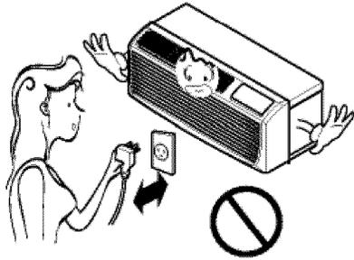
**Do not damage or use an unspecified power cord.**
