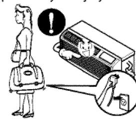
**Do not operate or stop the unit by inserting or pulling out the power plug.**
