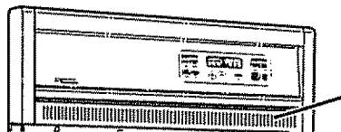
Oven Vent Location
