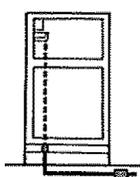
Through floor to basement cold water pipe
