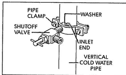
**5.** Fasten shutoff valve to cold water pipe with pipe clamp. Be sure inlet end is solidly in 3/16" drilled hole in water pipe and washer is under pipe clamp. Tighten packing nut. Tighten pipe clamp screws carefully and evenly so washer makes a watertight connection. Do not overtighten or you may crush copper tubing, especially if soft copper tubing is used. Now you are ready to connect the copper tubing.
