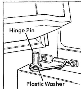
**(c)** Before tightening the top hinge screws, make sure the top of the door is level with the cabinet top and the space between the doors is equal across the entire front. Do not overtighten these screws—tighten them until they are just snug, then turn them in another one-half turn.
