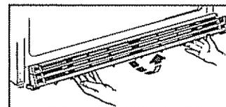
To replace the base grille, line up the clips on the back of the grille with the openings in the baseplate and push the grille forward until it snaps into place.
