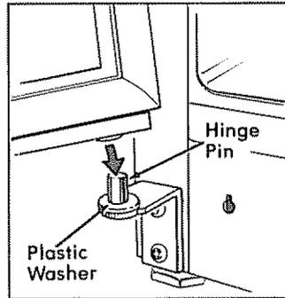
**(b)** Insert the pin on the center hinge into the socket in the top of the door. Note: The center hinge must be turned over as shown when mounted on the left side.
