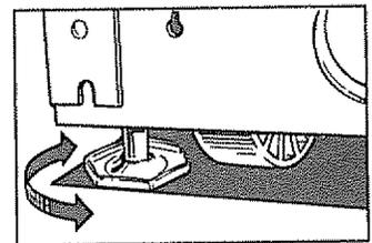
**Rollers** next to the leveling legs enable you to move the refrigerator away from the wall for cleaning. Turn the legs counterclockwise until the weight of the refrigerator is transferred from the legs to the rollers. After rolling the refrigerator back into place, turn the legs clockwise until the legs again support the refrigerator.
