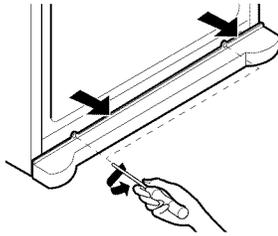
2. Turn the leveling leg clockwise to raise that side of the refrigerator or counterclockwise to lower it. It may take several turns of the leveling leg to adjust the tilt of the refrigerator.
