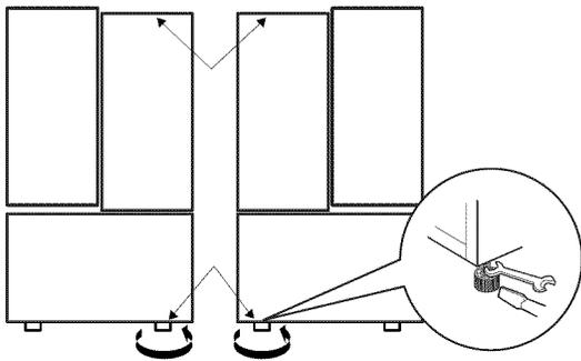
Level the refrigerator by using an 11/16 inch (18mm) wrench or a flat blade screwdriver. Turn the leveling legs counterclockwise to raise or clockwise to lower the height of the front of the refrigerator.
