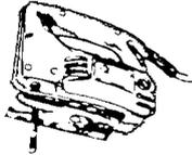
Saber saw (for cutting vent holes for roof or wall venting)
