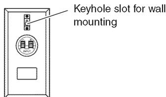
To mount the center speaker horizontally, use the two keyhole slots shown to hang each speaker on two screws that are securely screwed into the wall.
