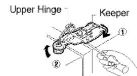
3) Remove the refrigerator compartment door by lifting it up.
