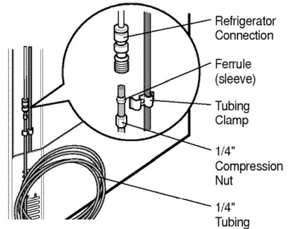
1. Remove the plastic flexible cap from the water valve.
