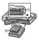
(B): Do not touch the connection terminals of the card.The card may be damaged if it is not fully inserted.
