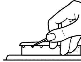
4. On the center and right burners, replace the burner cap, making sure the alignment pins on the cap are properly aligned with the burner base.
