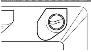
After changing the water filter cartridge, reset the water filter status display and indicator light by pressing and holding the **BUTTON** for 3 seconds.
