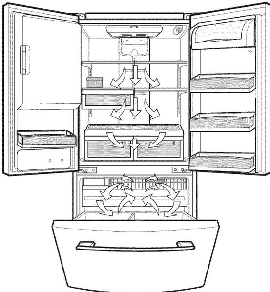
**Do not block any of cool air vents** with food packages. If the vents are blocked, airflow will be interrupted and temperature and moisture problems may occur.
