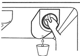
**NOTE:** There will be water in the cartridge. Some spilling may occur through the hole at rear bottom side of cover. You may use a cup or something like that to prevent spill water drop into food.
