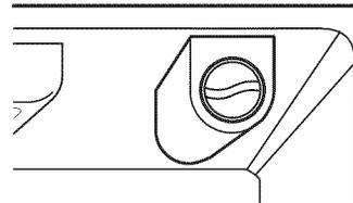
5. Turn the shutoff valve on (house valve).
