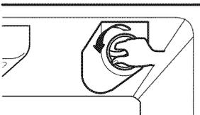
When the cartridge is removed, it will click out of place.
