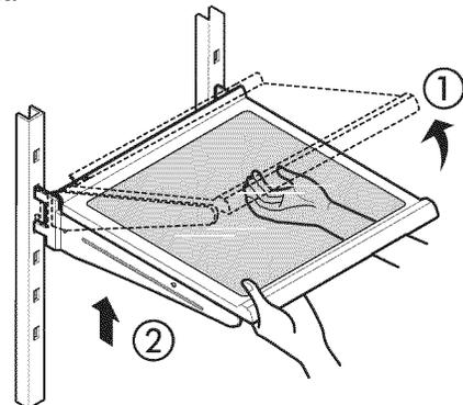
**To replace a shelf** Tilt the front of the shelf up and guide the shelf hooks into the slots at a desired height. Then lower the front of the shelf so that the hooks drop into the slots.
