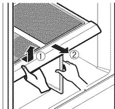
**⚠ WARNING:** Be careful when handling glass cover since glass is not attached to cover.
