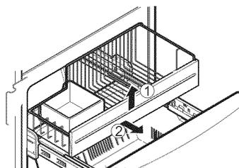
2. To Install, pull both rails out to full extension. Hook the basket supports into the rail tabs and push to the back of compartment.
