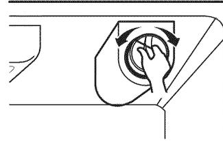
If you can't turn the filter from side to side, it isn't fully inserted. Push it in firmly and twist it into place. You will hear it click into place.
