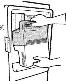
\* Avoid touching the automatic shut off arm when replacing the ice bucket.
