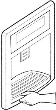
Tilt up the front of tray slightly and snap the ribs into the holes to reinstall the tray.
