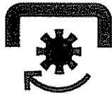
ATTACHMENT CLUTCH ENGAGED
