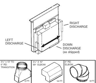
The system will operate most efficiently when the ductwork does not exceed 40 feet of equivalent duct. The chart above, shows equivalent feet of elbows and transitions. The number of feet of straight 3½" x 10" or 6" duct plus the equivalent feet of elbows or transitions to be used should equal 40 feet or less.
