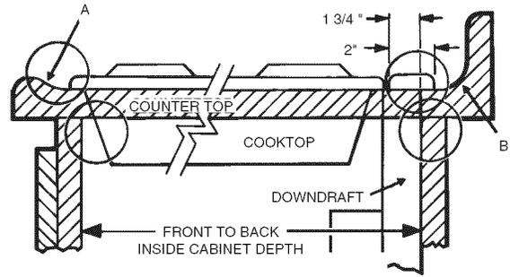
Refer to the cooktop installation instructions for dimensions of cooktop, countertop cut-out, and cabinet requirements. The 2830 and 2836 can be installed in most standard 30" and 36" wide cabinets.
