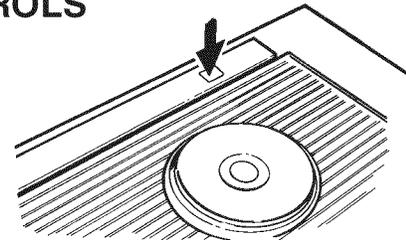
Turn the downdraft blower ON by pressing down on the activating switch. The air vent will rise.
