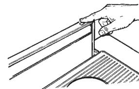
Turn the downdraft blower OFF by pressing the activating switch again. The air vent will go down and the blower will shut OFF.
