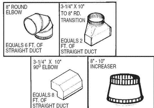
3. The system will operate most efficiently when the ductwork does not exceed 40 feet of equivalent duct. The illustrations, above, shows equivalent feet of elbows and transitions. The number of feet of straight duct plus the equivalent feet of transitions and/or elbows to be used should equal 40 feet or less.
