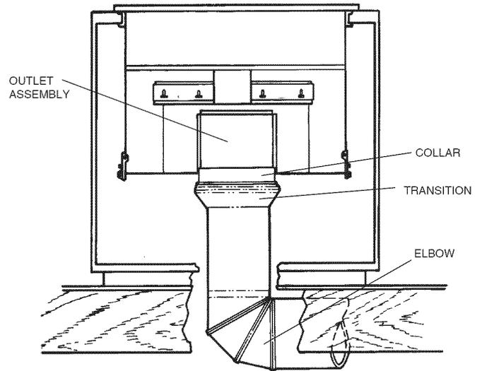
1. Cut hole in cabinet as well as holes in wall or floor as necessary.
