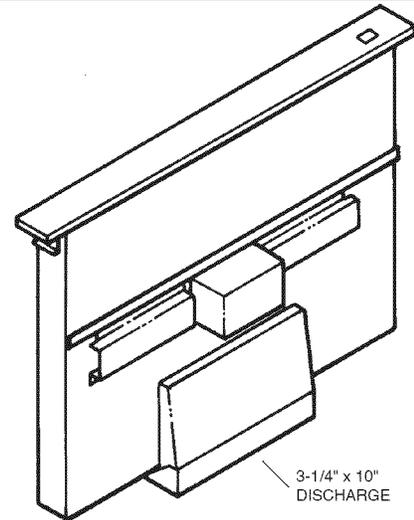
1. This downdraft blower system is most efficient when used with 10" round ductwork. Use a combination of elbows and transitions (shown below), closest to the downdraft, in order to get from 3" x 10" to 10" round as soon as possible.
