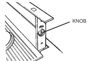
The blower can be turned ON or OFF and its speed can be adjusted with the recessed knob on the right side of the air vent.
