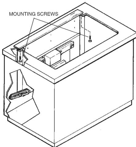
1. Set downdraft into opening. Extend leveling brackets to floor of cabinet so downdraft sits straight. (Note: Leveling brackets can be removed and re-attached in other positions. Bottom flange may have to face inward in tight cabinet installations.)
