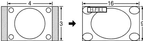
Enlarges the 4:3 image horizontally to the screen's side edges. The side edges of the image are cut off.
