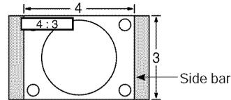
Standard (Note that "Image retention" of the side bar may occur from displaying it for a long time.)
