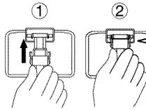
Insert it firmly until the tabs on both sides click into place.
