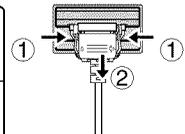
Keep pushing both side snaps and pull down
