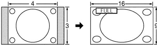
Enlarges the 4:3 image horizontally to the screen's side edges. (Recommended for anamorphic picture)
