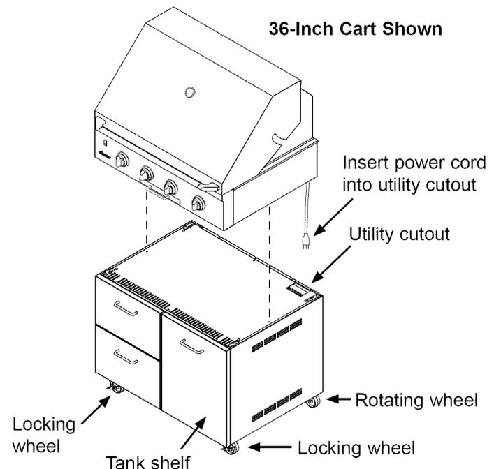
4. Center the unit on the cart, making sure to line up the threaded mounting holes under the bottom of the grill with the holes in the top of the cart.
