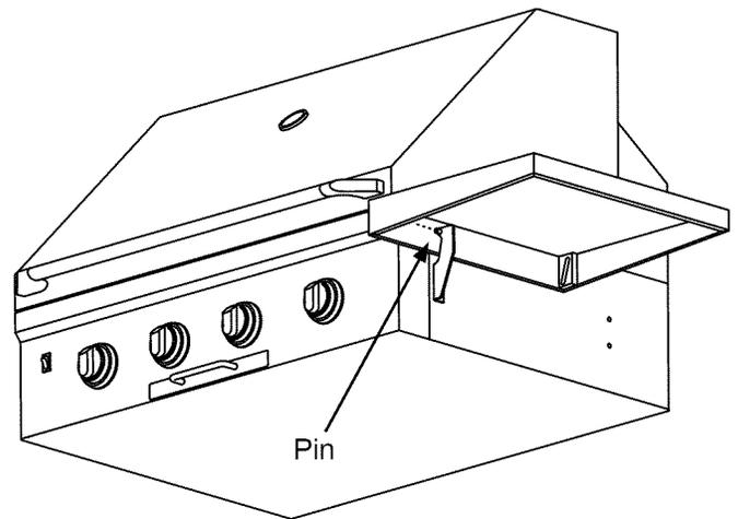
3. While holding the shelf in place, insert the pin on the back mounting bracket into the slot on the back side of the shelf.
