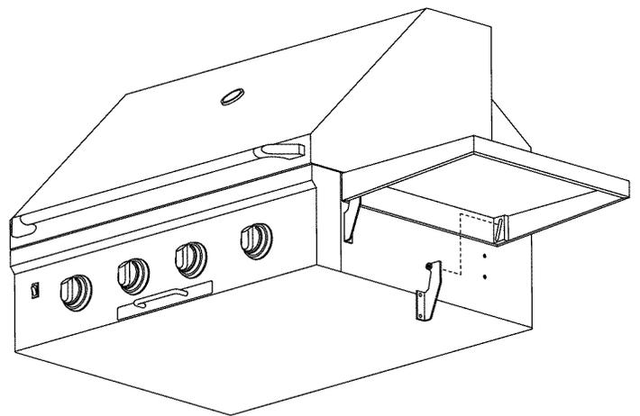
4. While holding the shelf and back mounting bracket in place, attach the back mounting bracket using two (2) of the provided button head fasteners and two (2) lock washers.
