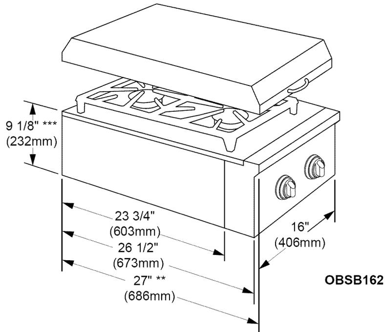
\*\* Total depth from back to front of knobs is 28 5/8" (727mm)
