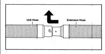
The extension hose has two tabs on the end that can be pushed into the slots and twisted to attach the two hoses together.
