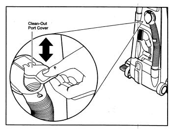
NOTE: Brush assembly will <u>not</u> turn if the hose is not fully inserted.
