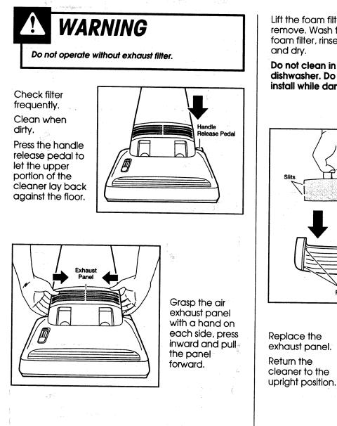
Lift the foam filter to remove. Wash the foam filter, rinse
