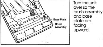
Lift the front wheels to gain easy access to the two latches. Locate the two latches which secure the base plate.
