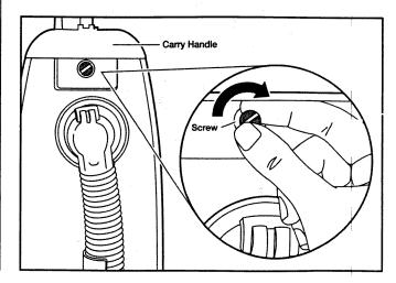
Using a screwdriver, tighten the screw.
