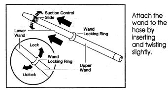
To achieve maximum reach (approximately 10 feet) with the attachments, add the crevice tool to the end of the wand by inserting and twisting slightly. Hose Suction Control Slide TO OPERATE SUCTION Telescoping Wand **CONTROL SLIDE** (Telescoping Wand) Crevice Tool When using attachments for cleaning draperies, small rugs with low pile and other delicate items, twist the Suction Control Lever
