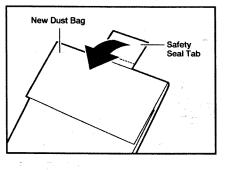
Fold the safety seal tab on the new bag away from the opening that fits on the dirt tube.
