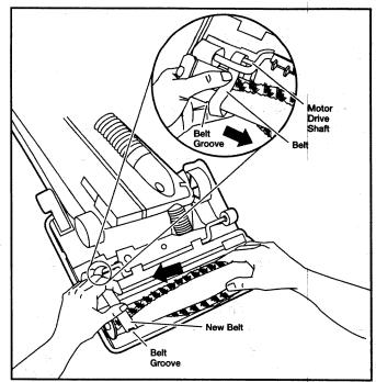
Loop the new belt on the motor drive shaft.
