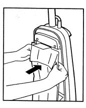
Position the bag cover so its positioning tab fits into the body positioning tab slot.
