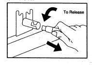
Pull the light bulb to remove.
