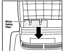
If the foam Motor Safety Filter located at the base of the bag cavity is dirty, remove it by pulling forward.
