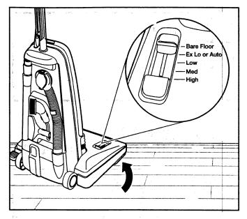
In this position, the headlight is off and the brush assembly does not revolve. This setting is recommended for cleaning hardwood and tile floors.
