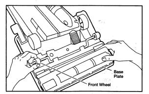
On the right side, lift the latch hook slightly to place the base plate into position. The base plate will not close unless the base plate is under the latch hook.
