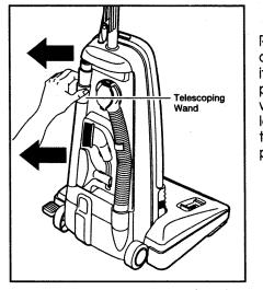
Remove the crevice tool from its storage position in the wand. Turn the locking ring to the **UNLOCK** position.
