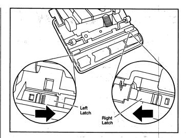
Slide latches toward the center of the unit to secure.
