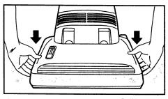
Replace the base cover over the base. Press down firmly so the cover snaps onto the base.
