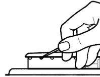
4. Replace the burner cap, making sure it is centered properly on the burner base.
