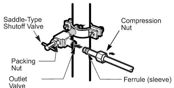
**NOTE:** Commonwealth of Massachusetts Plumbing Codes 248CMR shall be adhered to. Saddle valves are illegal and use is not permitted in Massachusetts. Consult with your licensed plumber.
