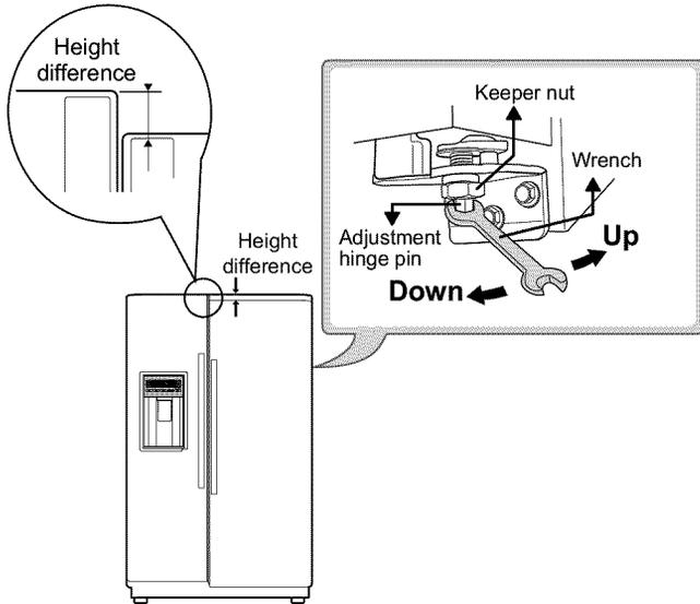
Using a 3/4" (19 mm) wrench, turn the keeper nut clockwise to loosen the keeper nut.
