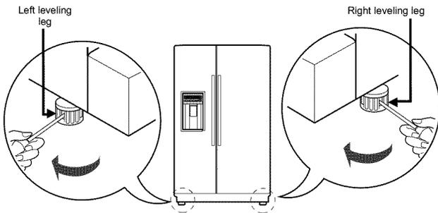
Raise the front of the refrigerator enough so the doors close freely when opened halfway. The refrigerator should slope  $\frac{1}{4}$ " (6.35 mm) to  $\frac{1}{2}$ " (0.127 mm) from front to back.
