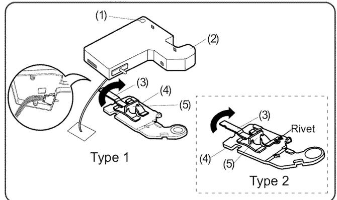
1. Open the door. Remove the top hinge cover screw (1).
