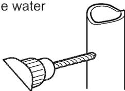
**NOTE:** The hookup line cannot be white, plastic tubing NDA tubing #49595 or 49499 or Cross Link Polyethylene (PEX) tubing.
