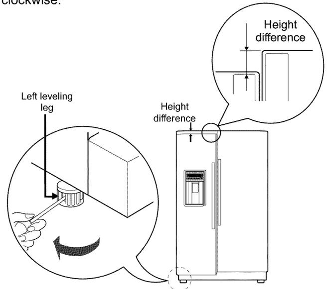
If the freezer compartment door is higher than the refrigerator compartment door, make them level by inserting flat blade screwdriver into the groove of the right leveling leg and rotating it clockwise.
