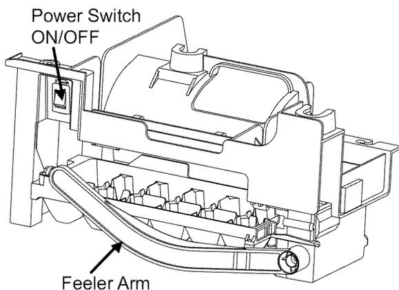
The icemaker will produce 12 cubes per cycle, approximately 140-150 cubes in a 24-hour period, depending on freezer compartment temperature, room temperature, number of door openings and other operating conditions.
