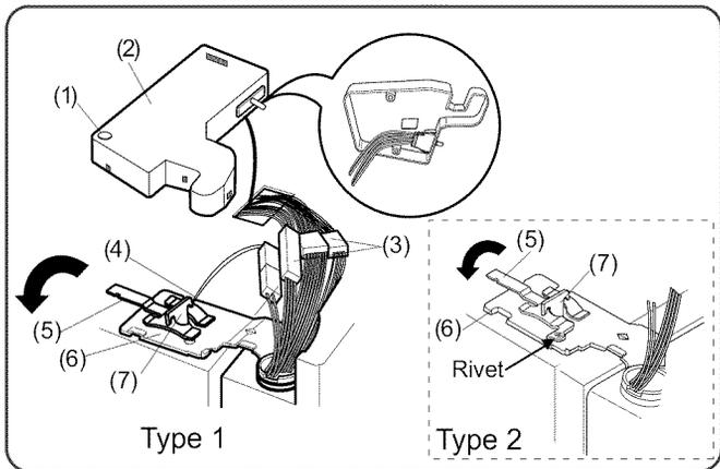
1. Open the door. Remove the top hinge cover screw (1).
