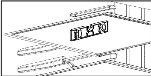
If your refrigerator is not level, insert a flat blade screwdriver into the grooves of the leveling legs (shown in picture below). Rotate legs clockwise to raise or counterclockwise to lower the front of the refrigerator.
