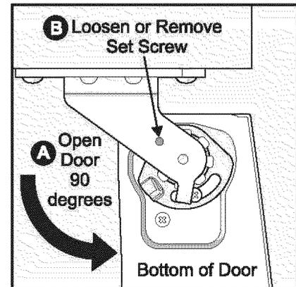
**Loosen/Remove Set Screw**
