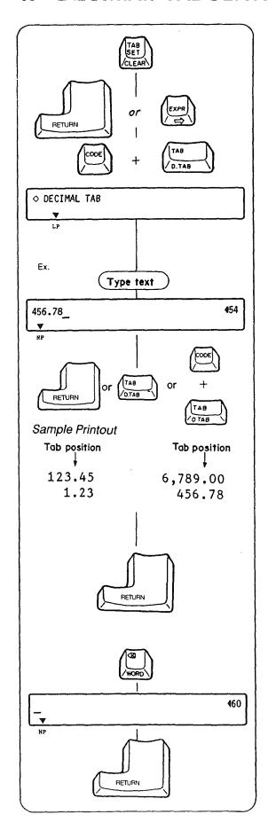
This function allows you to do statistical typing easily. All numbers are automatically aligned by their decimal points.
