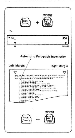
This function sets a temporary left margin, which eliminates the need for constant tabbing or spacing after each carrier return.
