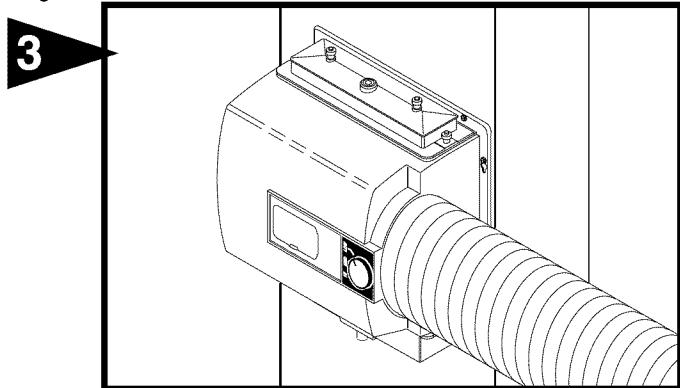
Cut out center section of template and 6" hole. Hang humidifier cabinet and insert remaining four screws. Tighten all 8 screws. Install connecting collar after drilling 1/8" holes for screws. Connect by-pass pipe to collar and humidifier cabinet. Using holes at top and bottom of humidifier bypass opening drill 2-1/8" holes through bypass pipe and screw by-pass pipe to humidifier cabinet.
