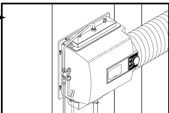
Connect drain hose to 5/8" spout on humidifier cabinet using hose clamp provided. Run 5/8" hose to suitable drain such as floor drain, sewer or laundry sink. Be sure hose has continuous slope and is not kinked at any point.
