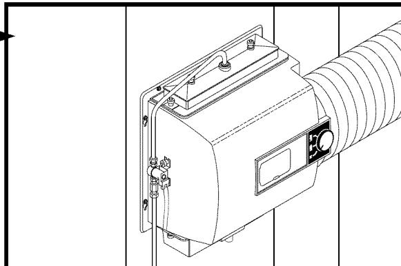
Attach solenoid valve to side of humidifier cabinet with flow arrow pointing up, using thumb nuts provided. Do not reverse brass fittings as valve will not function if flow is reversed. Assemble distributor tube so that it is directed into the center opening of the distributor trough cover. Connect 1/4" water supply tube to brass filter at inlet of solenoid. DO NOT USE PLASTIC TUBING IN CONTACT WITH ANY HOT PLENUM SURFACE OR DUCT. IF USING PLASTIC TUBING, USE TUBE SUPPORT PROVIDED.
