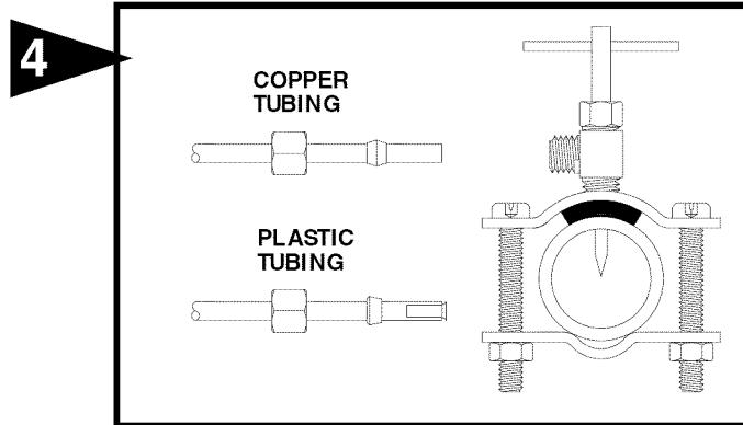
Mount the self tapping saddle valve on either a cold or a hot water pipe. A side or top mount is best to avoid clogging from pipe sediment. Connect 1/4" O.D. tubing to the saddle valve. Copper tubing requires a brass compression nut and brass sleeve. Plastic tubing requires a brass insert inside the tubing, a plastic sleeve on the outside with a brass compression nut.
