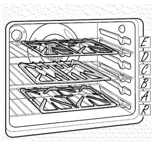
The oven has 5 rack positions. Place the gray porcelain-coated racks in positions "R", "B" and "D" for self-cleaning the grates. Place one grate each on the oven racks from side to side.
