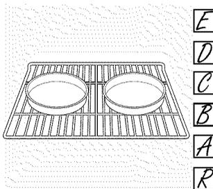
When baking on a single rack, use the rack position from the chart for your type of food. Baking results will be better if baking pans are centered in the oven as much as possible.
