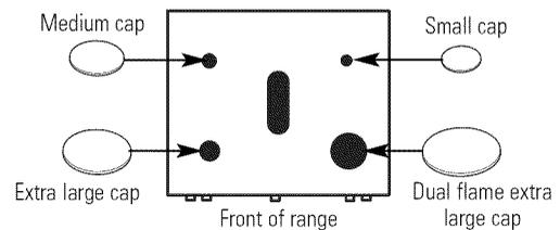
Make sure that the heads and caps are replaced in the correct locations.
