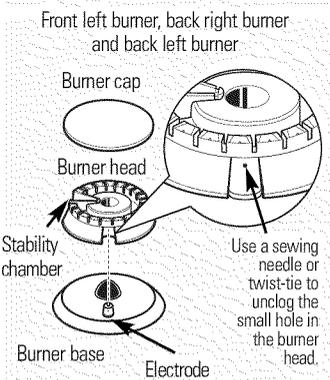
Make sure the slot in the burner head is positioned over the electrode.
