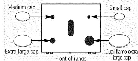
Make sure that the heads and caps are replaced in the correct locations.
