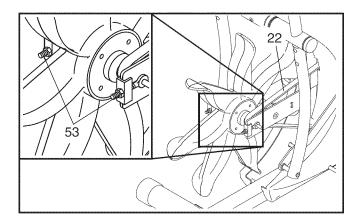
**See the drawing at the left.** Make sure that the Fan (5) is straight, and then reattach the Left Guard (13), tighten the Guard Fasteners (35), and reattach the Guard Clips (76).
