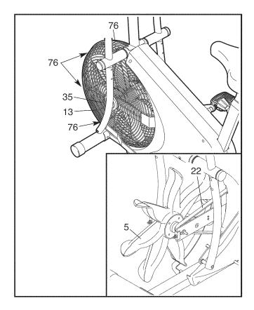
If the Belt (22) needs to be adjusted, first loosen the right Guard Fastener (not shown). To tighten the Belt, turn the M6 Nuts (53) clockwise; to loosen the Belt, turn the M6 Nuts counterclockwise.
