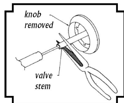
**Figure 14-1 - Adjusting brass burner low heat setting.**
