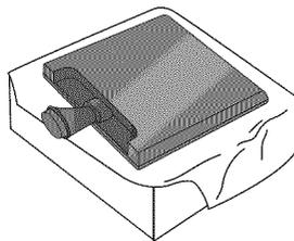
2. Turn the Stand Base Lock through 90° to separate the Stand Base from the Stand Body.
