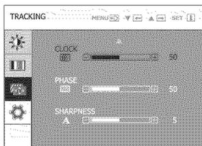
**CLOCK** To minimize any vertical bars or stripes visible on the screen background. The horizontal screen size will also change.
