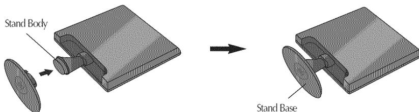
3. Turn the Stand Base Lock through 90° to fix the Stand Base to the Stand Body.
