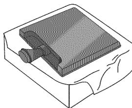
2. Assemble the Stand Base into the Stand Body in the correct direction.
