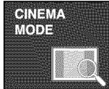
**CINEMA MODE** To focus on the moving picture selected. This function adjusts the brightness of areas other than the user-selected area to provide an environment and image quality optimized for videos or moving picture on the web browser.
