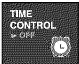
**TIME CONTROL** To notify the user of a specified time. This function notifies the user that a user-specified time (1 or 2 hours) has passed, which is done by displaying the Alarm OSD and the LED blinking.
