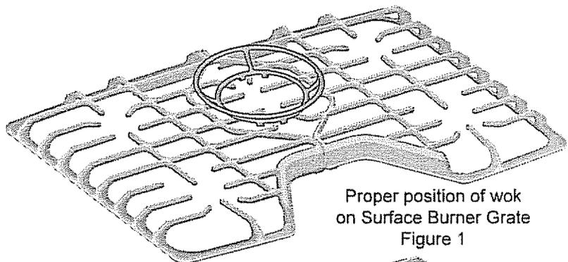
Proper position of wok on Surface Burner Grate
