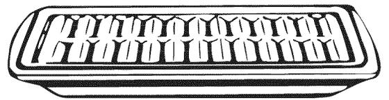
The broiler grid is designed to prevent smoking and spattering by trapping juices (fats and oils) from foods in the lower part of the broiling pan.
