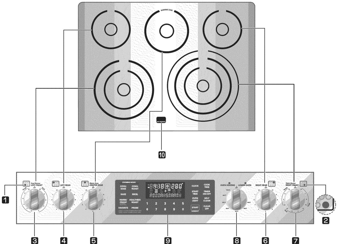
**1 SURFACE COOKING AREA LOCATOR :** Identify which element the knob controls.
