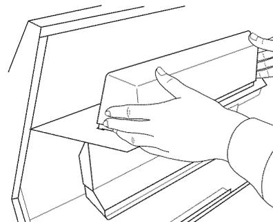
2. Screw light bulb into socket. If you are using a 25-watt light bulb as a night light, screw into right-hand socket.
